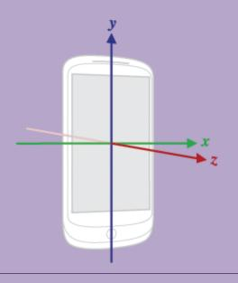
• Gyroscope - a device that measures orientation in terms of yaw, roll, and pitch.
